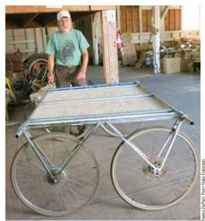
Dr. Cogger, Washington State University, designed these lightweight harvest carts, which can be pushed down the row by workers and keep produce boxes off the ground.
